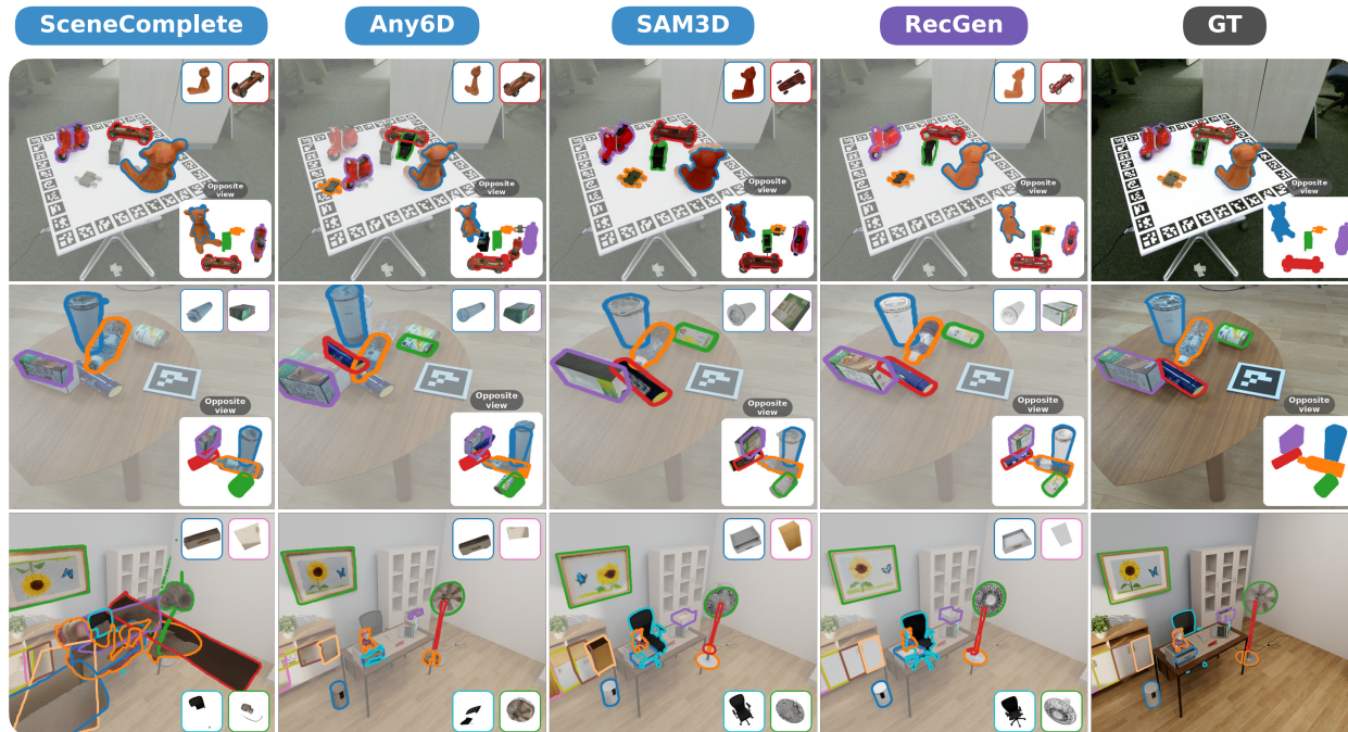
Figure 1 RECGEN generates full reconstructions of complex occluded scenes from single or multiple RGB-D images, enabling robust generation of digital twin replicas of real-world environments. Our model recovers occluded geometry of both objects and parts, is robust to imperfect sensor depth, and handles object symmetries — challenges that most recent baselines struggle to address.
