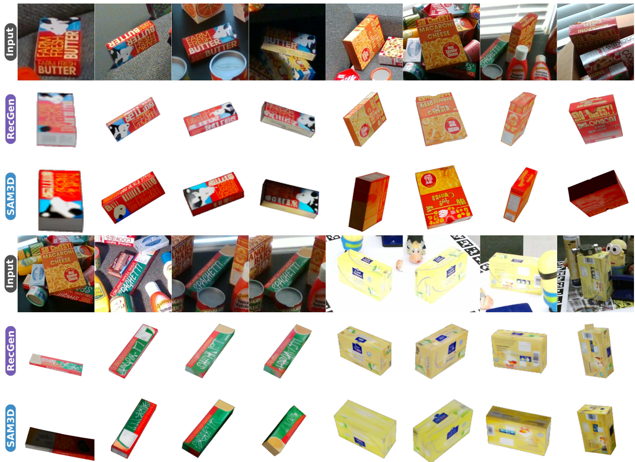
Figure S3 Appearance generation for objects with symmetric shapes. Top block: HOPE objects 3 and 12). Bottom block: HOPE object 25 and HB object 29. For each block: input image (top), REC GEN reconstruction (middle), SAM3D reconstruction (bottom). REC GEN produces textures consistent with the ground-truth orientation across diverse symmetric objects.
