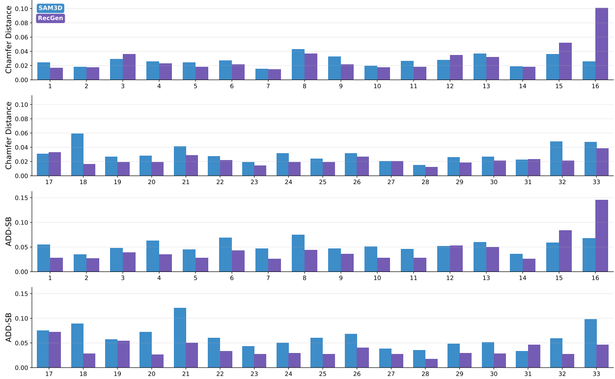
Figure S2 Per-object comparison on HB dataset. Chamfer Distance (top two rows) and ADD-SB (bottom two rows) for each of the 33 HB objects. Lower is better. RECGEN (purple) outperforms SAM3D (blue) on 26/33 objects for shape and 29/33 for pose, while both have one outlier object on which they perform significantly worse than on other objects.
